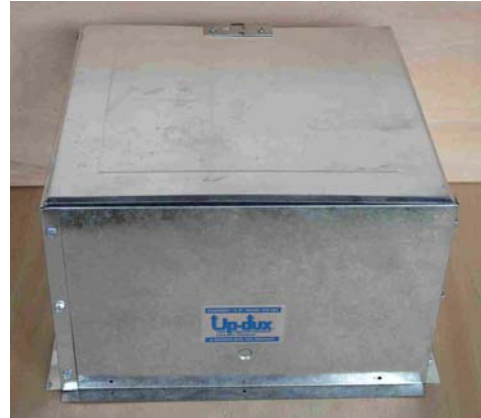
Figure 5. Up duct. The grill of this up-duct is secured to the ceiling while the upper portion extends into the attic. Of course, insulation should be packed around the duct, but not on top. This model includes an insert to prevent air exfiltration during the heating season.
